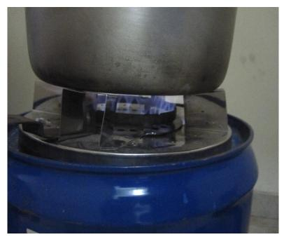
using a water boiling test showed that the stove consumes 400 grams of fuel per load. It is able to produce combustible gases in just a minute from the time of fuel ignition. Moreover, one and a half liters of water can be boiled within 13 minutes. The figure in the right side shows the
