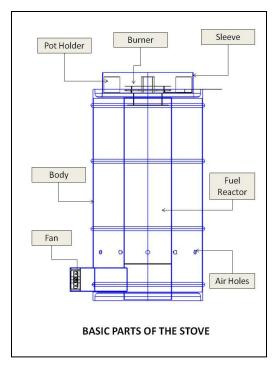
and the burner; (c) the fan, which uses DC 12 volt, 2 watt supplies the required air to gasify rice husks. The flame coming out of the burner is bluish in color, which indicates a very clean gas. It has low black carbon emission of about 50 ug/m<sup>3</sup> and below. The CO<sub>2</sub> emission is about 0.6 kg CO<sub>2</sub> per kg rice husks.
